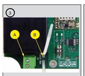
Connect the 230V (A) and secure the powercable with the tie-wrap (B). Apply the power.
