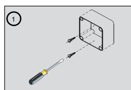
Mount the repeater in the area covered by the transmitter. Under no circumstances the transmitter should be directly mounted on a metallic surface.
