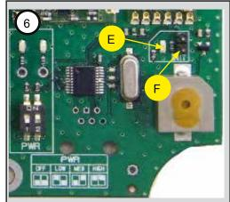
In "initialisation" mode, the LED (E) is on. To switch the repeater back in Init mode, short the two pins (F) for 3 seconds.
