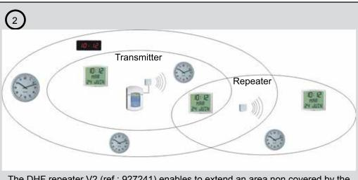
The DHF repeater V2 (ref.: 927241) enables to extend an area non covered by the main DHF transmitter.
