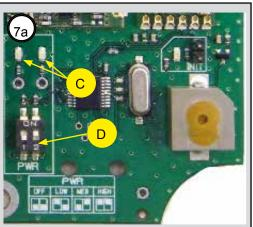
You can adapt the transmission power with two DIP switches (D). LEDs (C) allow you to check your setting.
